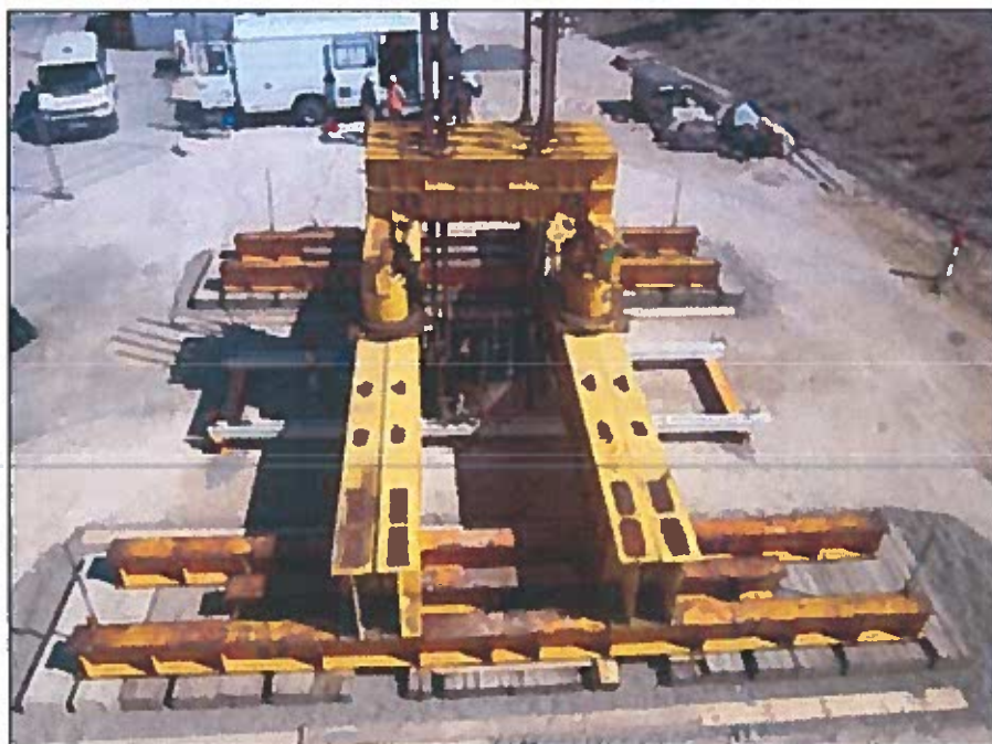
Photograph of 'H' Shaped Testing Rig (© Bauer Renewables Ltd)
