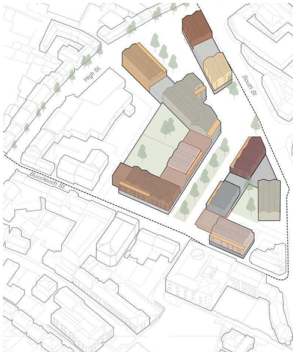
Axonometric View of proposed buildings showing Massing, Setbacks, Terraces & Dual Aspect Views
