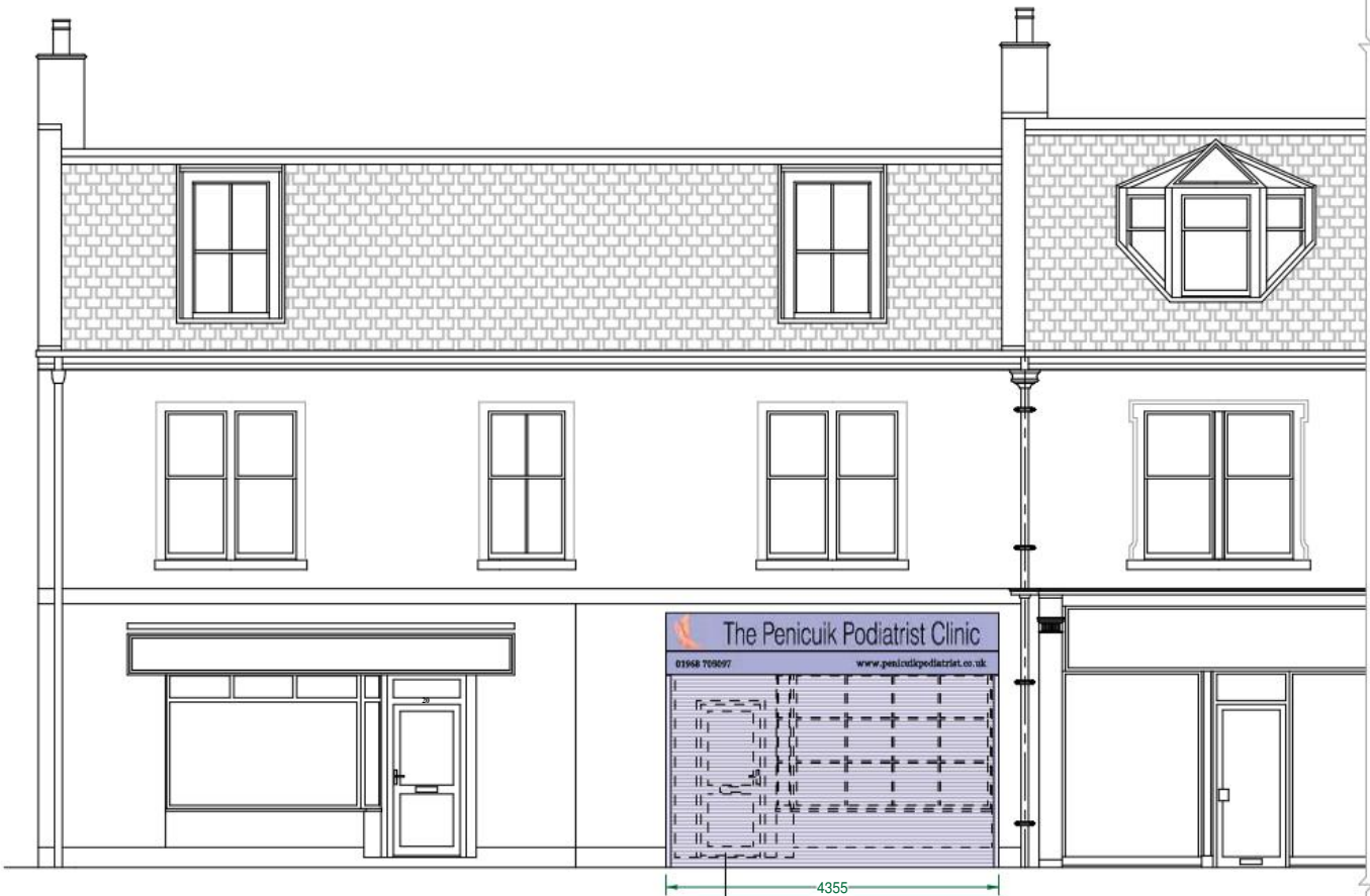
PROPOSED EAST (JOHN STREET) ELEVATION 1:100 SCALE
