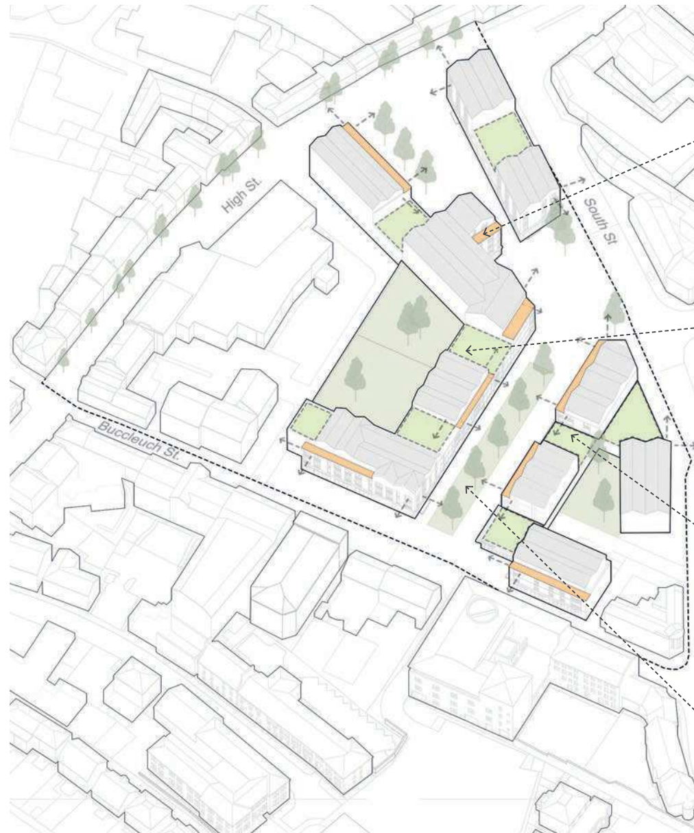
Axonometric View of proposed Housing with Pitched Roofs, Setbacks, Terraces & Dual Aspect Views
