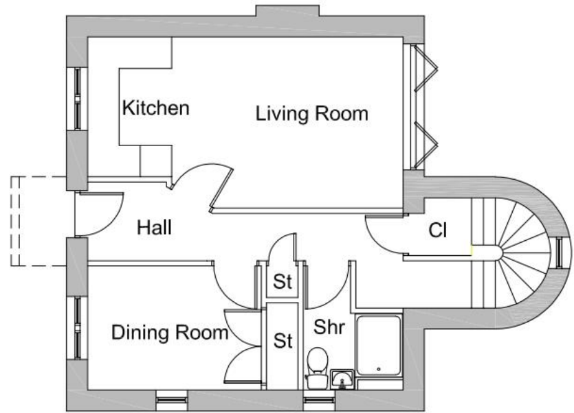
HOUSE TYPE 1 [gifa 74.68sq.m.] Ground Floor Plan
